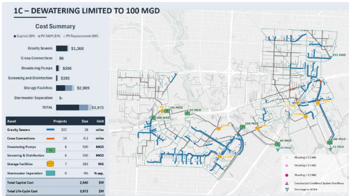
Figure 32. Alternative 1C – Dewatering Limited to 100 MGD
